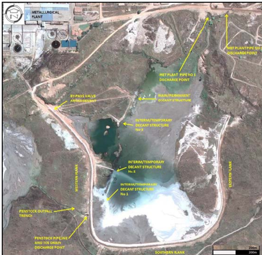
Figure 35: Layout of the Kamoto Interim Tailings dam
