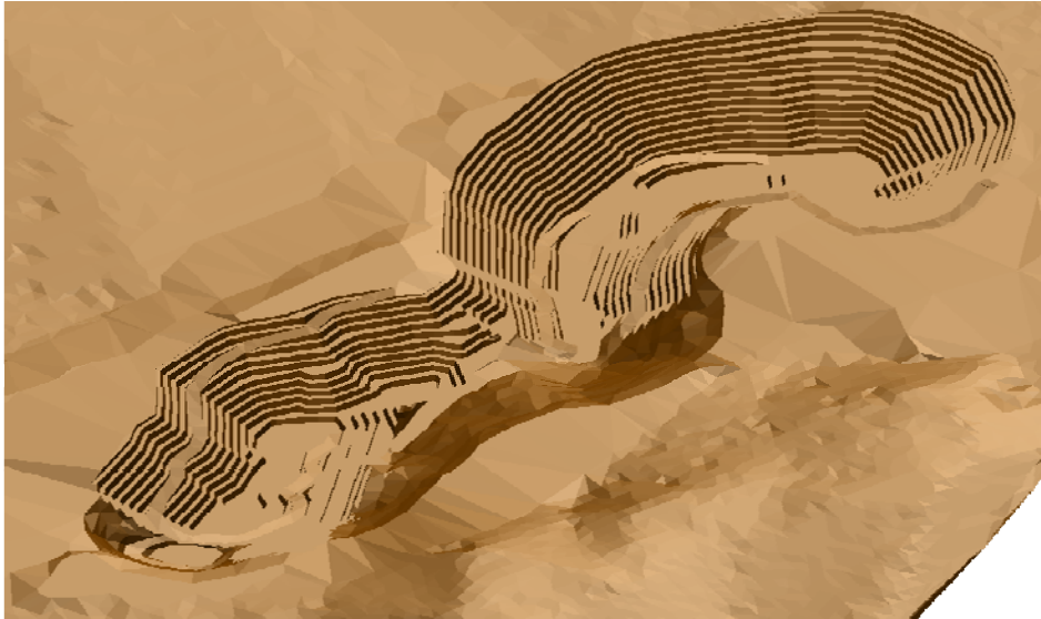
Figure 26: Mashamba East Open Pit Design
