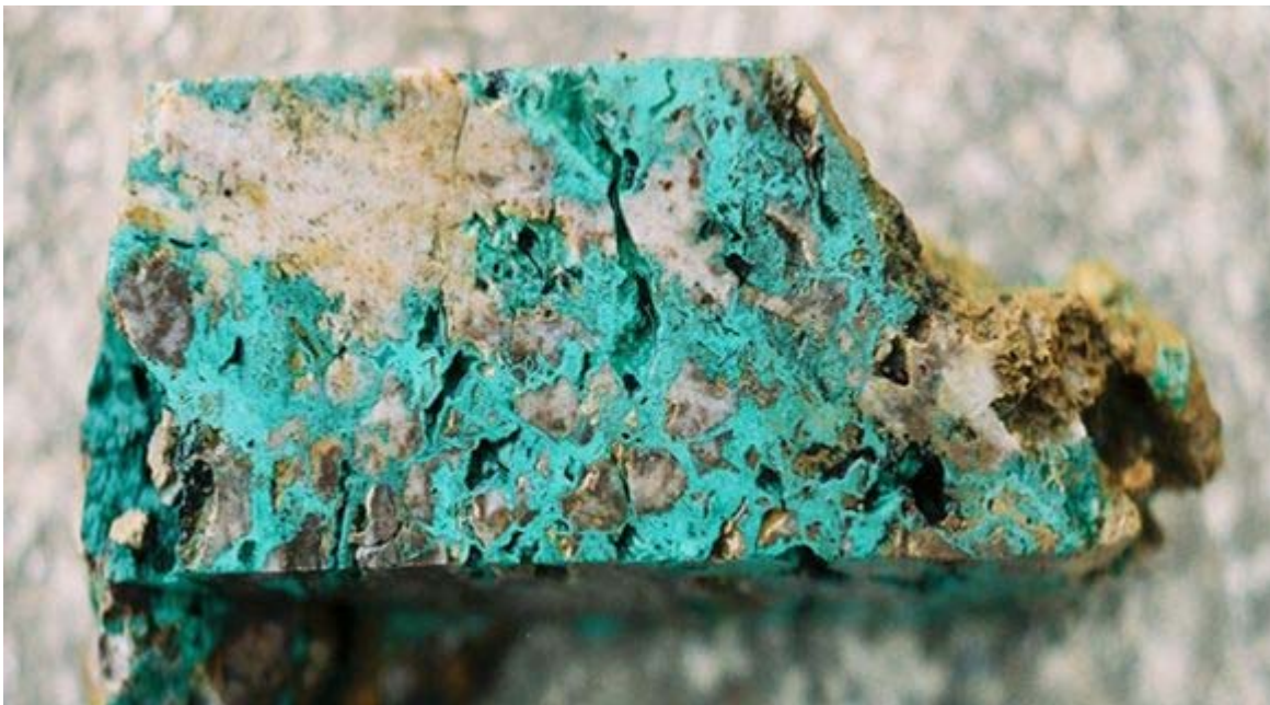
Figure 9-5 NQ sized DDH core from DIK 171 (Mashamba East) showing weathered RSC with secondary enrichment of malachite in the network cavity structure. Core length is 10cm
