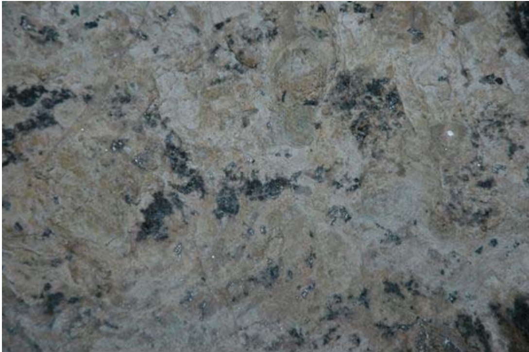
Figure 11-1 Recrystallised pink feroan dolomite of the lower metre of the RSC, showing the abundance of visible shiny crystals of carrollite ( \text{Co}_2\text{CuS}_4 )
