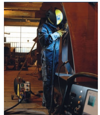
The manual MIG/MAG welding process
