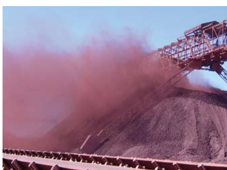
Chemical dust suppressants are being used at Sishen mine to reduce exposure to dust and nuisance to neighbours
