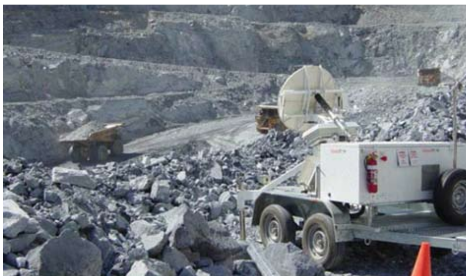
Slope stability at Callide mine is monitored by radar
