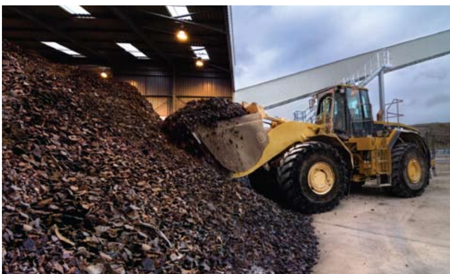
Rubber chips from tyres that can not be retreaded or reused have become an important carbon neutral fuel for the cement kiln at Tunstead
