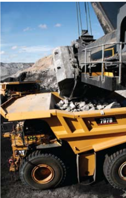
At Dawson mine in Australia fuel consumption for larger dump trucks was reduced from 0.750 litres/tonne (105 l/hr) to 0.696 litres/tonne (240 l/hr). This represents a 7% improvement
