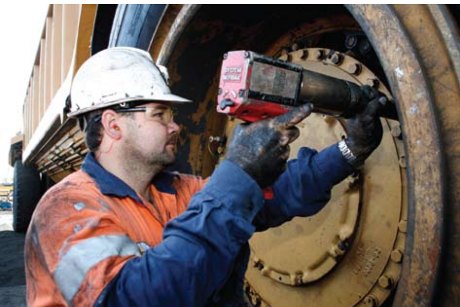
Fitter Konrad Kirkman at Capcoal mine in Australia checks the tension on the wheel rim bolts of a large haul truck. Maintenance of tyres and wheels has increased tyre life and slashed costs
