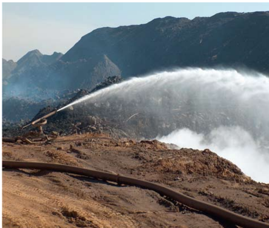
A water cannon is used to address spontaneous combustion and cool down blasted overburden before this is removed to expose the coal seam
