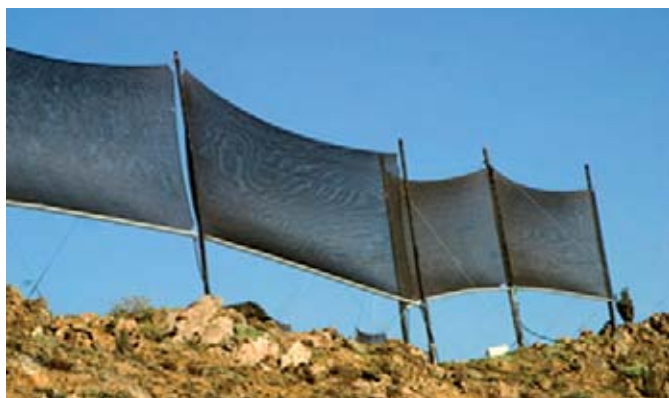
Left: A mist trap for harvesting water at Chanaral in Chile's Atacama desert.
