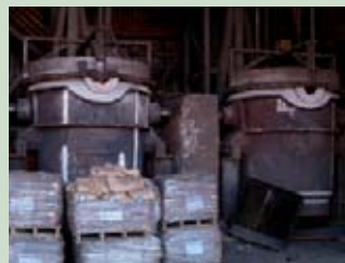
Left: To save energy during off-peak times, the Namakwa Sands smelter uses only one ladle heater.
