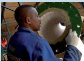
Left: The fitment of pre-engineered ceramic tiles into a pipe at Kram Engineering's Sebenza operation.
