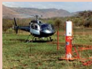
Left: Recent MagSQUID tests in South Africa to find and characterise buried orebodies.
