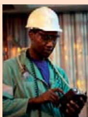
Left: Control of exposure at source requires ongoing monitoring of exposure. A worker is shown here with dust measuring equipment.
